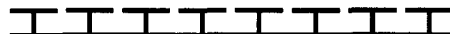
Figure 1 Cross-sectional view of a high-impedance, textured metal ground plane, consisting of metal protrusions on a flat conducting surface.
