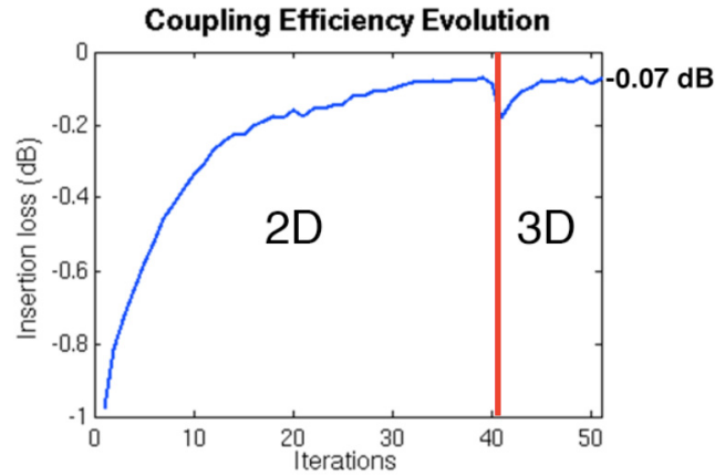
Fig. 3. Coupling efficiency evolution during the optimization. The switch from 2d to 3d FDTD is visible at iteration 41. For comparison, the previous record of ref [3]. was -0.13\text{dB} and required 1500 simulations.
