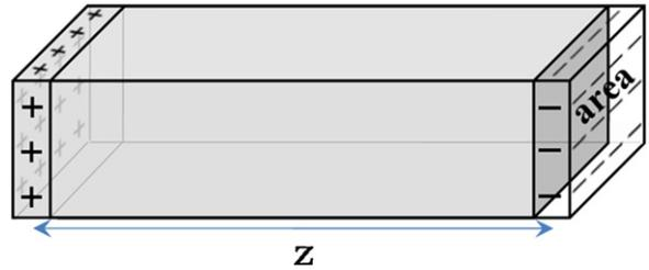
Fig. 1. The displacement of electrons in a rectangular metal bar leads to a Coulombic restoring force, and oscillations at the bulk plasma frequency,  $\omega_p = \sqrt{(nq^2/\epsilon_o m)}$ .
