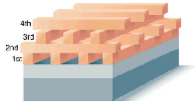
The excellent report by Noda *et al.* (2) represents a watershed in photonic crystal research. The authors demonstrate unprecedented optical rejection  $>10,000$  in a GaAs photonic band gap structure. All of the key requirements for photonic crystal-based optoelectronics are demonstrated in this work.
