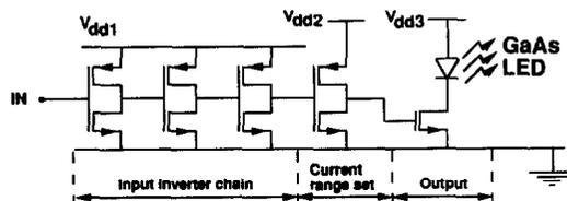
Fig. 4. The schematics of the driver chip to be used with the epitaxial liftoff LEDs.
