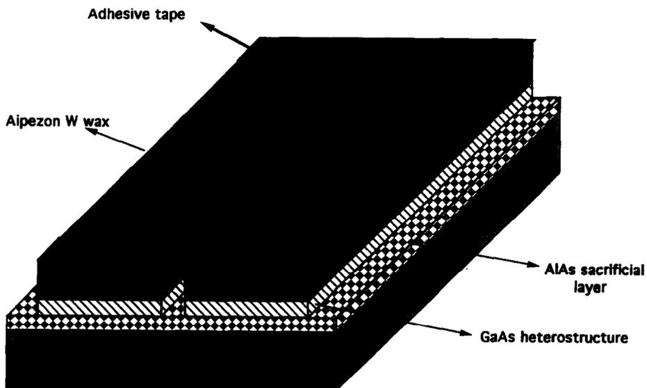
Fig. 8. The illustration of the sample after wax patterning. HF can attack the sacrificial AlAs layer through the streets which have been patterned in the wax.
