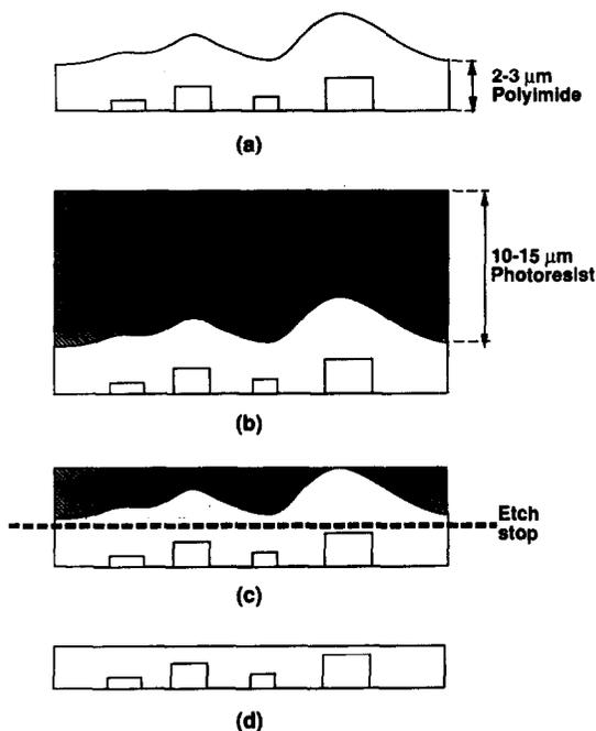
Fig. 3. The sequence of the plasma etch back process: (a) polyimide spin; (b) thick photoresist spin to obtain a planar surface that is independent of the substrate topography; (c) since the etch rate ratio of PR to PI is close to 1, it is possible to carry the etching down to the etch stop point without degrading planarity; (d) final planarized surface.
