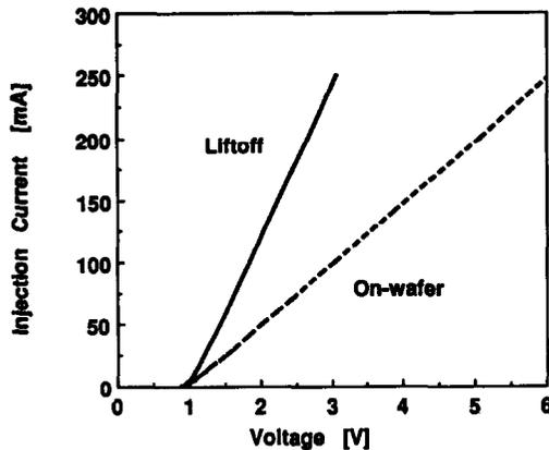
Fig. 11. Typical  $I$ - $V$  characteristics of a liftoff LED and on-wafer LED, as described in Fig. 10.
