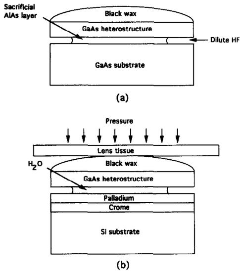
Fig. 1. The illustration of ELO process: (a) separation of thin film from its substrate; (b) bonding of the thin film onto another substrate that is coated with Pd.
