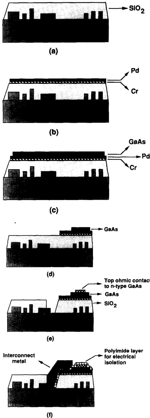
Fig. 5. The sequence of the post-processing steps to fabricate GaAs LEDs: (a) planarized silicon chip; (b) Cr/Pd deposition; (c) GaAs film bonding; (d) patterning of GaAs and underlying metal layers; (e) top *n*-type ohmic contact metallization followed by contact hole openings for the *p*-type GaAs to silicon circuit interconnect; (f) polyimide spin for LED sidewall isolation and final metallization.
