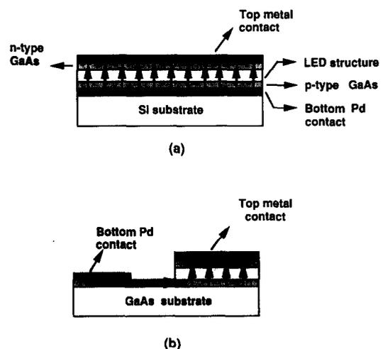
Fig. 10. The liftoff LEDs do not require a *p*-type metallization step (a). Electrical injection to the same LED structures grown on semi-insulating substrates requires additional mesa etching (b). Clearly the resistance of the vertically injected LEDs, (a), is lower than for the laterally injected LEDs, (b).
