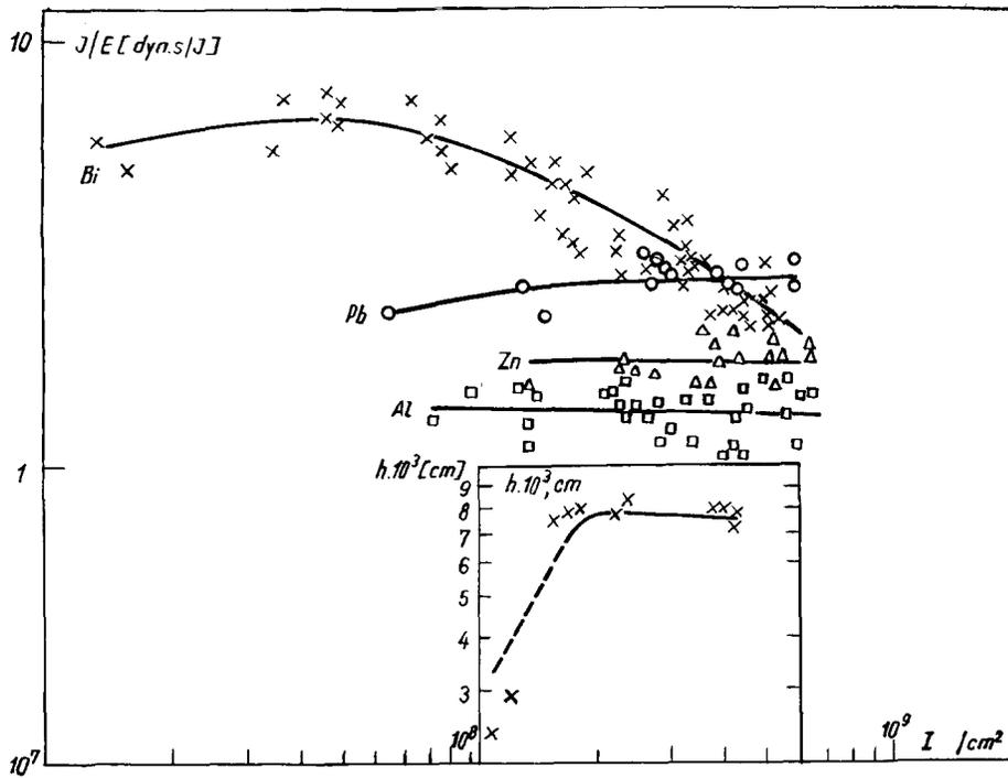
Fig. 2. Specific recoil impulse,  $J/E$ , for Bi, Pb, Zn and Al and crater depth,  $h$ , for Bi, versus incident intensity on target,  $I$ .
