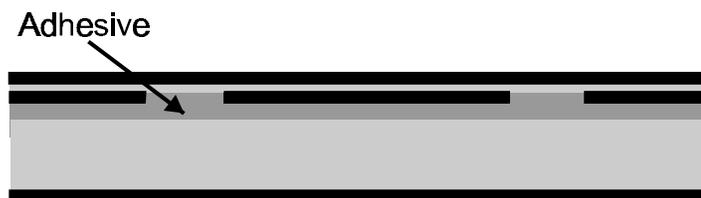
**Figure 4.2.3 Two sheets bonded with an adhesive**
