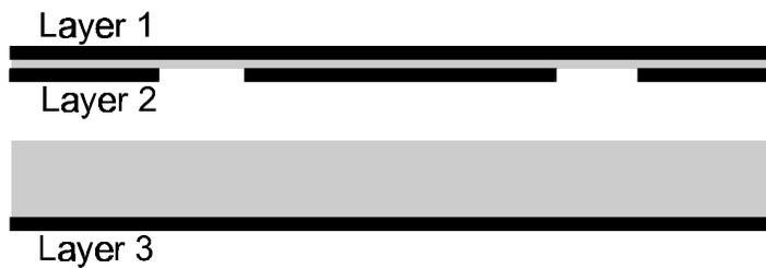
**Figure 4.2.2 Inner layers patterned by etching**
