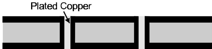
**Figure 4.1.3 Plated copper forming vertical interconnections**
