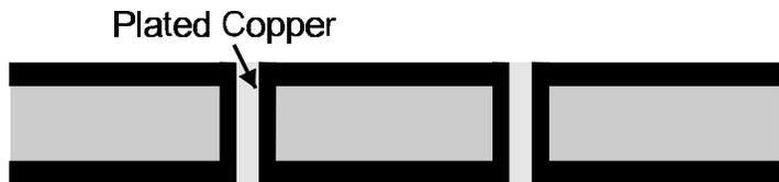
**Figure 4.1.3 Plated copper forming vertical interconnections**
