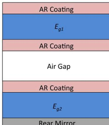
Figure 3.6: Case (3); a dual bandgap solar cell with an air gap intermediate mirror, with perfect antireflection coatings and a perfect back mirror.
